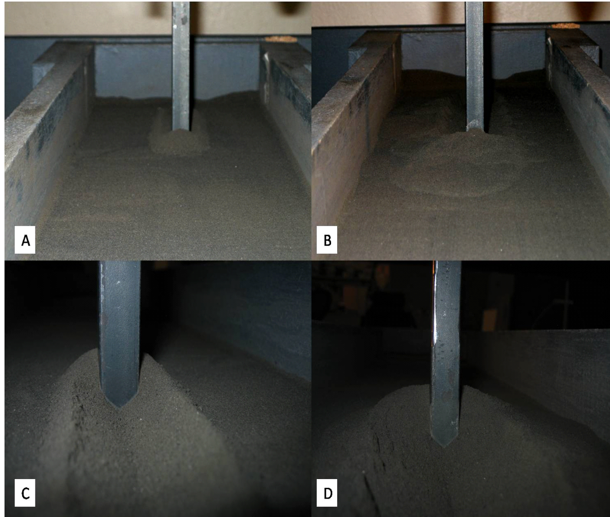
Square rod pushing through JSC-1A lunar simulant (A) The back view at a cut depth of 0.635 cm. (B) The front view at a cut depth of 6.985 cm. The surcharge is about 1.25 cm. (C) The back view at a cut depth of 0.635 cm. (D) The back view at a cut depth of 6.985 cm.
