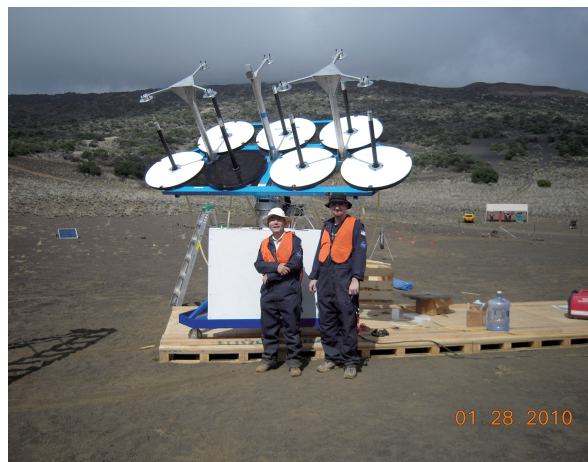
Figure 2. The fully integrated solar concentrator system.
