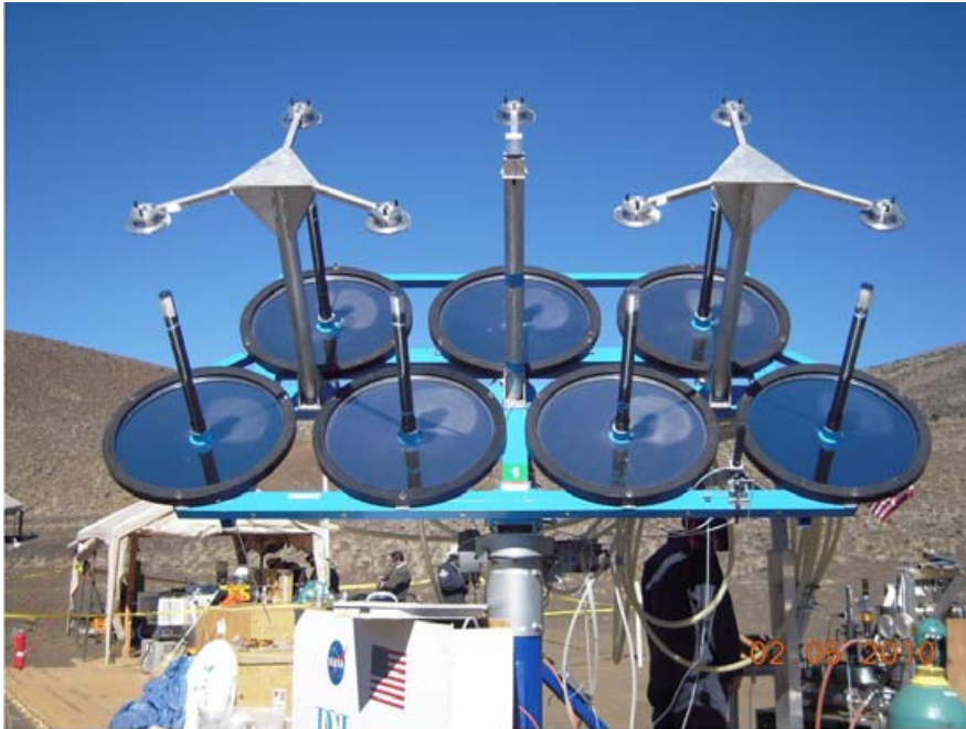
Dust Deposit on the Primary Concentrators
