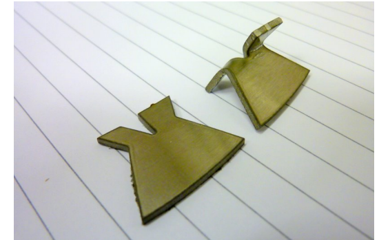
Blade in Chris Dreyer's inclined centrifuging test rig
