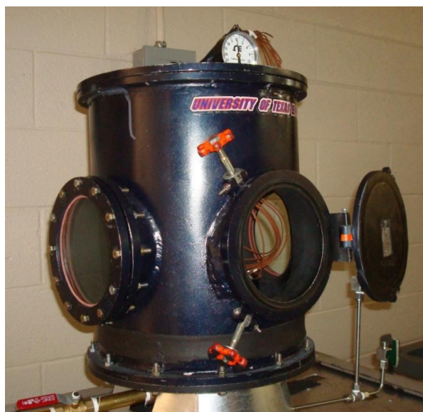
Fig. 1. A photograph of the reaction chamber.
