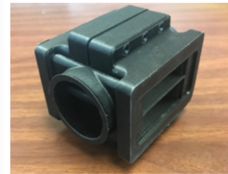
Rapid cycle adsorption pump 'one-plate' assembly design (L); RCAP 'one-plate' test-printed in plastic
