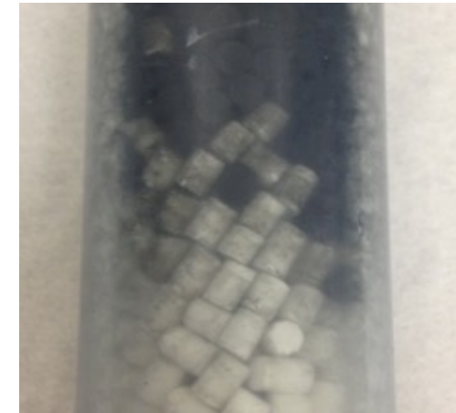
Post-vibration testing showing catalyst dust migration
