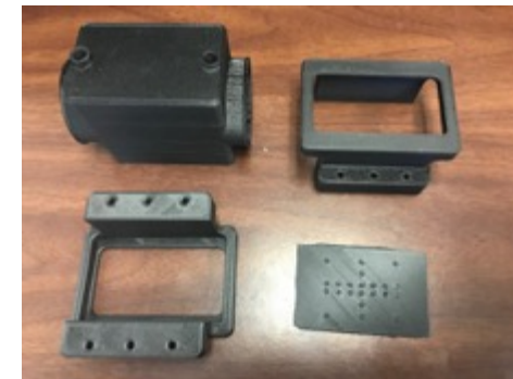
Rapid cycle adsorption pump 'one-plate' assembly design (L); RCAP 'one-plate' test-printed in plastic
