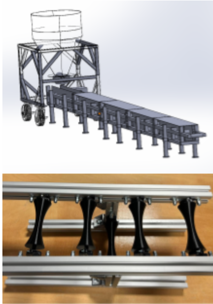
Fig. 1: Horizontal transport system render (top) and downscaled mock-up (bottom)
